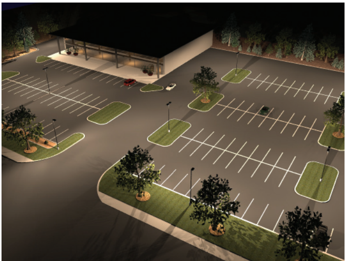
Prevail A40 LED 14 Fixtures = 2,002 Total watts
