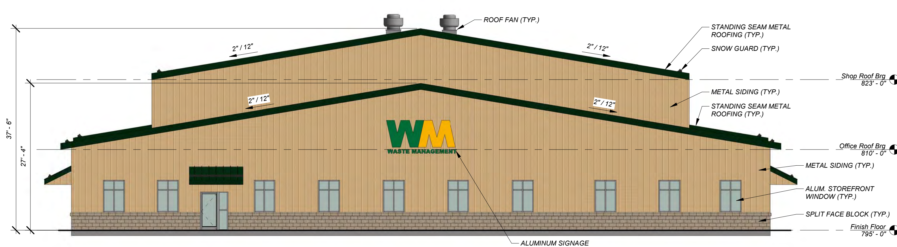
1 East Exterior Elevation 3/32" = 1'-0"
