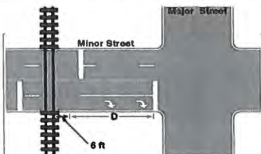
Figure 4C-9 Warrant9, Intersection Near a grade Crossing (One Approach Lane at the Track Crossing)
