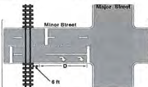
Figure 4C-9 Warrant9, Intersection Near a grade Crossing (One Approach Lane at the Track Crossing)
