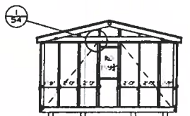
2 ENDWALL FRAMING WINDOW
