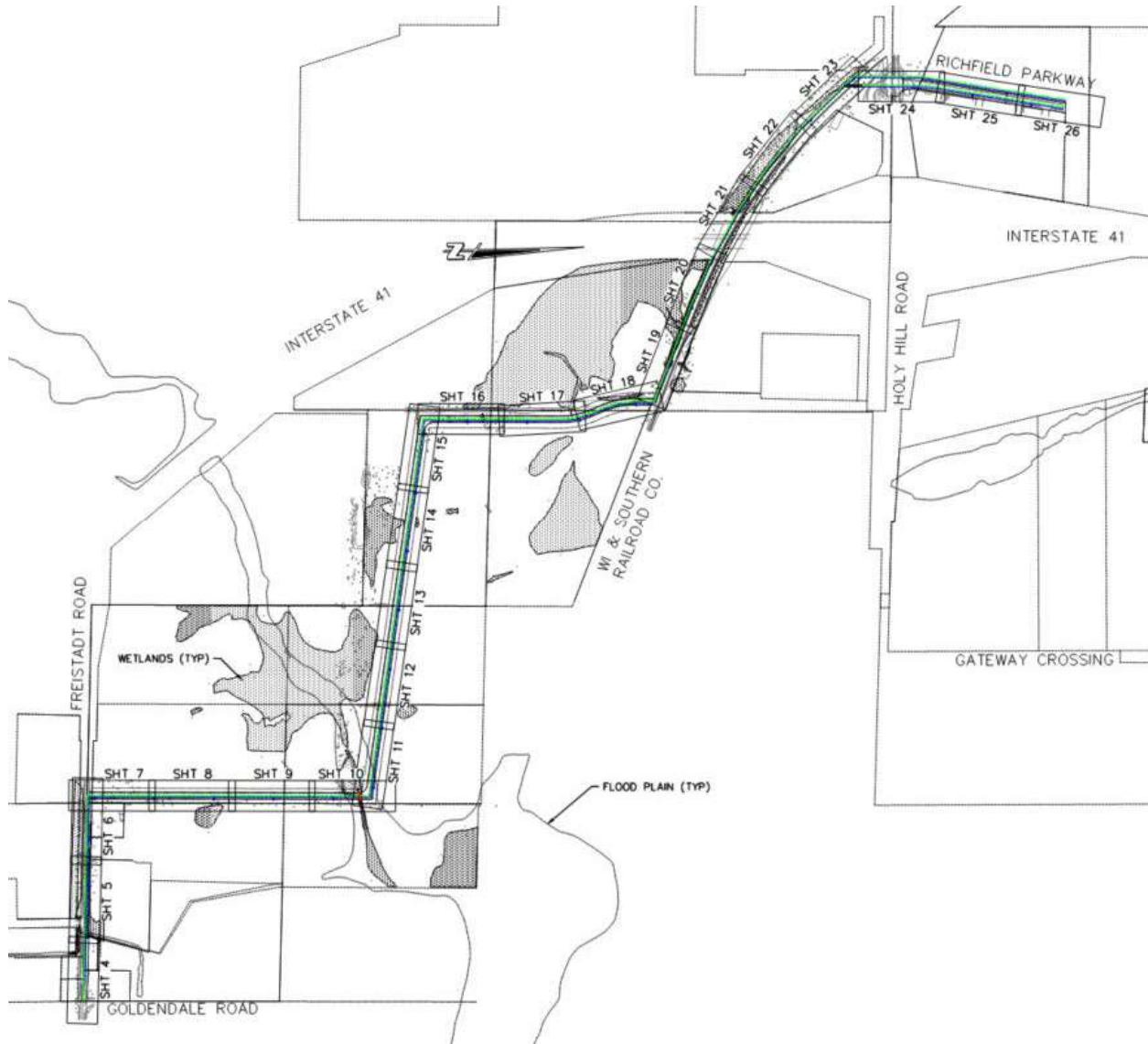
Figure 9 Preliminary Route of Sewer and Water Extensions to Serve the Richfield SSSA
